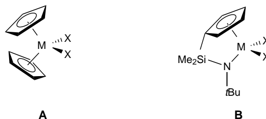
Scheme 1. Group 4 metallocenes ( A ) and constrained-geometry catalysts ( B ).
